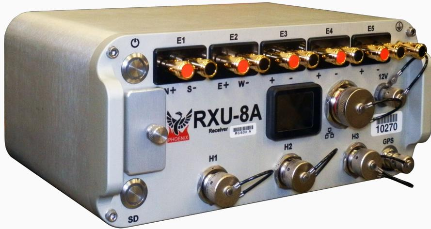
Designed with flexibility in mind, the RXU-8A can be used as a regular MT receiver, where the extra electric channels can be used to acquire a redundant recording on the same site or to acquire an adjacent site.
